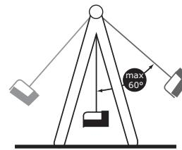
**WARNING!** Pushing the seat too strongly forward, especially above the indicated maximum angle (see figure), is dangerous and could lead to tipping the seat over. As a result the child could fall out of the seat!
